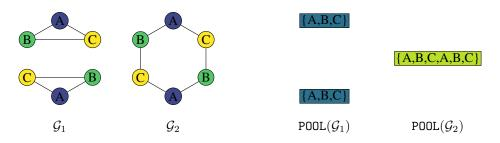
Figure 1: Two WL-indistinguishable graphs  $\mathcal{G}_1, \mathcal{G}_2$  which can be distinguished after pooling as in Theorem 1. Clustering cycles maps  $\mathcal{G}_1$  to a two supernode graph, while it maps  $\mathcal{G}_2$  to a single supernode graph.
